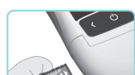
2. Hold the test strip by the end with the horizontal raised lines. Insert the test strip into the test strip slot until it will go no further. (When the test strip reaches the correct position, the analyzer will beep.)
