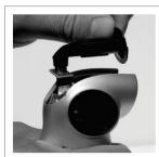
Lift the breath tube to access the sensor module.
