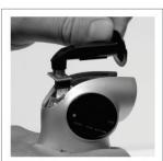
Re-attach the breath tube directly on to the sensor. Make sure the front opening is aligned.
