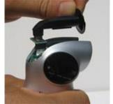
Re-attach the breath tube directly on to the sensor. Make sure the front opening is aligned.
