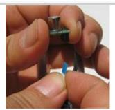
Remove the cable from the slot underneath the sensor module.
