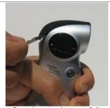
Use a flat, sharp tool to carefully open the top cover.
