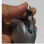
Carefully raise the sensor module from the body. Do NOT detach the cable from the body.
